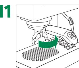
Insert filter basket into porta-filter and insert into group head, reattach cup-holder grid
