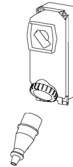
Disconnect the general sectioning device and provide to protect the plug with proper systems
