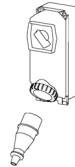
Disconnect the general sectioning device and provide to protect the plug with proper systems
