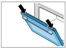
3. Open the appliance door fully and push in the direction of the appliance.
