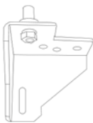
10. Refit the bottom hinge pin to the bottom hinge which was turned.
