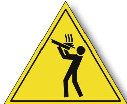
The label ISO 3864-1 here on the side must be stuck on a visible surface, 1,6 mt height from the ground.
