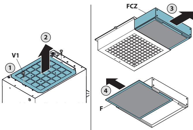
**The zeolite-carbon filter and lower dust filter cannot be washed.**
