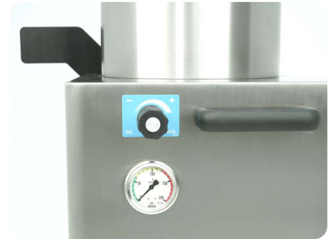
Speed control & pressure gauge.
