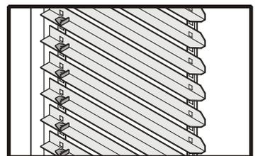
First slide bars into the rear clip-in upright at the desired height and then hang in position at the front.
