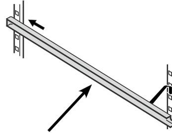
Suspend the rails at the desired height, by inserting into the rear clip-in strip first and then clipping in at the front.
