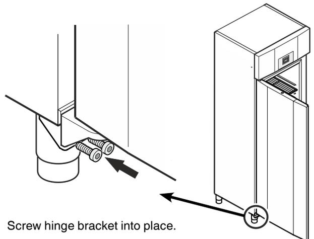
12. Screw hinge bracket into place.
