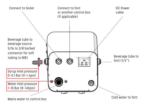
if using chiller add chiller connector here (3/4" to pushfit elbow) and connect to chiller output. also slelect chiller present page 14.
